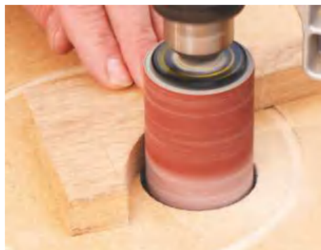
STEP 18. Tidy up the curves of each bracket with a sanding drum or spokeshave, making sure you keep edges square
